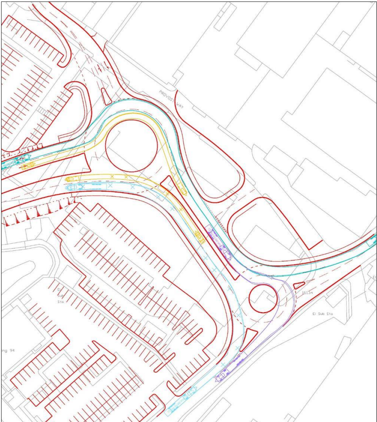
Figure 3.2: Swept Paths - AAR / Provost Way
